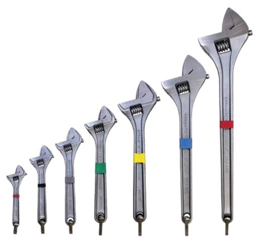
Our Adjustable Wrenches for Working At Height feature shackle attachment points. The versatile wrench fits a wide range of different sized nuts and bolts. The head is tilted 15° for a 30° deflection angle when flipped and the reduced nose thickness allows for better access. The Adjustable Wrench for Working At Height is made from hardened Steel.
